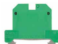
EK 2.5/35 Single-level ground terminal - Positive ground Termination - screw-down feet make contact to both sides of rail
